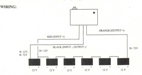
\*\*CAUTION\*\* 200V output possible. Care must be used when installing controller. First, connect black wire to B- (input-, output-); second, connect orange wire (output+) to B+ (72V); third, connect red wire (input+) to B+ (12V).
